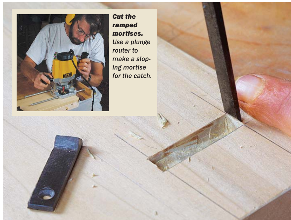
Pare the mortise to the length of the catch using the catch as a guide. Pare less vigorously as you come close to the desired width.
