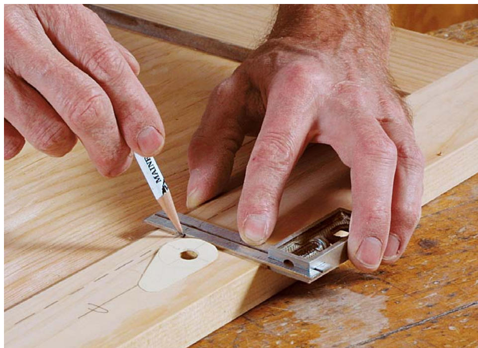
Lay out the mortise. With the knob hole drilled in the center of the stile, use a cardboard cutout to determine the spinner's placement. Then mark the mortise ⅜ in. larger than the spinner itself.
