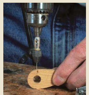
Predrill for the pin. To avoid splitting the spinner, drill a hole for the escutcheon pin.
