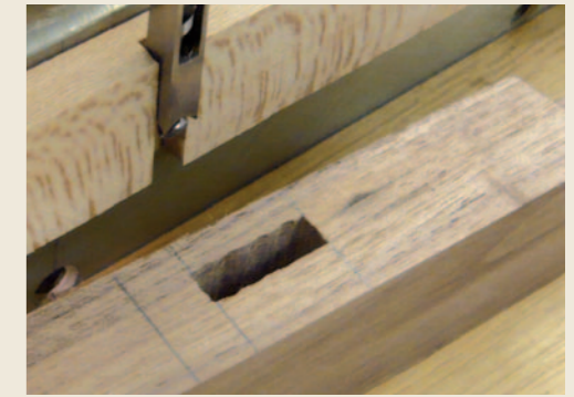
Pic.4 Because the auger inside a hollow chisel has only one edge it can drift outwards and cut beyond the edge of the mortise
