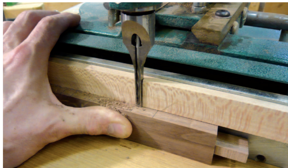
Pic.3 Each slat on Eric's Hinta chair (top) is tenoned into the rails or the back leg. Eric has a trick for paring mortises without the auger (above, see right)
