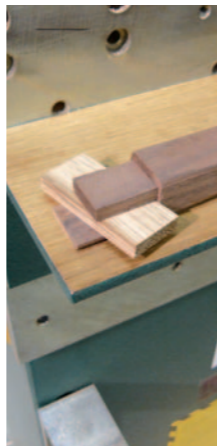
Pic.2 Eric uses a spacer the thickness of the tenon shoulder (above) to set the fence accurately (left). A notched bar (below) helps align the mortise and holds down the workpiece (below)
