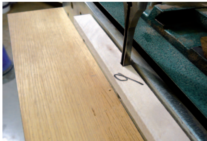
Pic.1 Eric has a notched stick (above) for setting the hollow chisel parallel to the fence. Why isn't this a standard feature?
