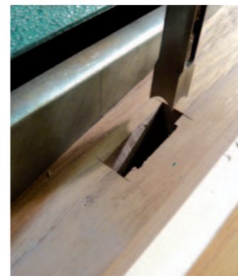
Pic.3 Each slat on Eric's Hinta chair (top) is tenoned into the rails or the back leg. Eric has a trick for paring mortises without the auger (above, see right)
