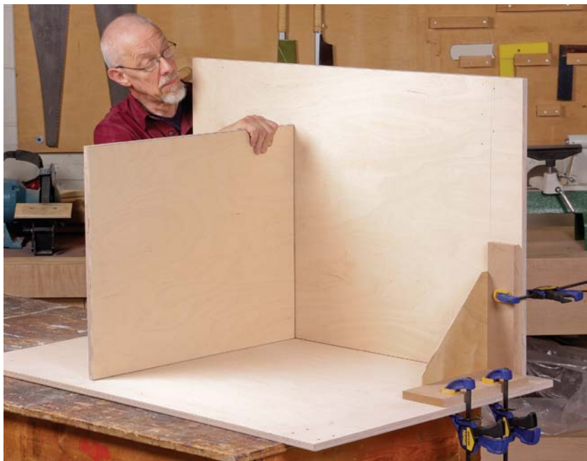
Get a third hand for assembly. White used a simple plywood corner block to hold parts still and square to one another while he drove in screws.
