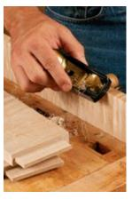
A champ at profiling. The block plane's small size gives it great flexibility in cutting chamfers or custom rounded profiles.
