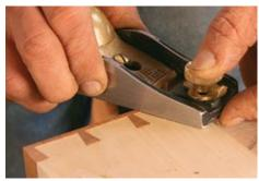
**Trim dovetails perfectly flush.** A low-angle block plane can bring the end grain of the pins flush with the surface of a drawer side.
