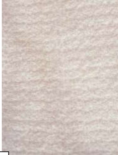
2 FELT FILTERS are comprised of dense layers of polyester fibers, which trap most of the finest dust, while letting air pass back into the room.
