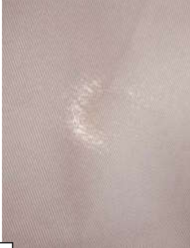
1 WOVEN BAGS are poor filters. The pinholes you see here allow the most hazardous fine dust to blow right back into your shop.
