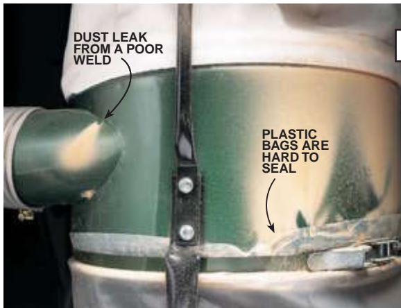
4 DUST LEAKS were common around bag flanges and duct welds. Plastic bags are a pain in the sitter to seal even when using spring clamps. Tip: A couple of 20-in. bicycle inner tubes can be stretched around the bag flange to help form a good seal for the bags. Silicone caulk can be used to seal any duct leaks.
