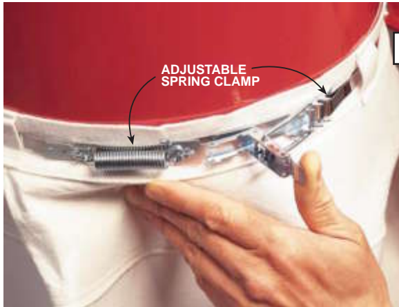
3 ATTACHING A BAG after it has been removed for emptying is a fact of life with single-stage collectors. Getting the bag off isn't so tough, but putting it back on can be a real challenge. We found adjustable spring clamps provide the best combination of seal and ease of use for single-stage collectors.
