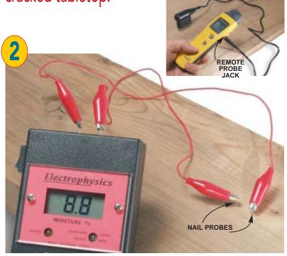
**External probes extend the reach of your meter.** External probes driven to the center of a board allow you to get a core reading in stock that's too thick for the pins built into the meter. The probes can also be left in a stack of green wood where readings can be taken to monitor the wood as it dries. Some meters have built-in jacks for aftermarket probes, but a pair of nails and alligator clips are an effective, low-cost alternative for all pin-type meters.
