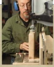
And adjusted the carriage for drift. After installing each blade, a test cut was made on a scrap block of wood to determine the angle of blade drift; then the carriage was adjusted to match the angle.
