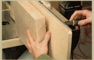
Then mounted the test blocks securely to the carriage. Each test block was screwed to the carriage before the test cuts were made.
