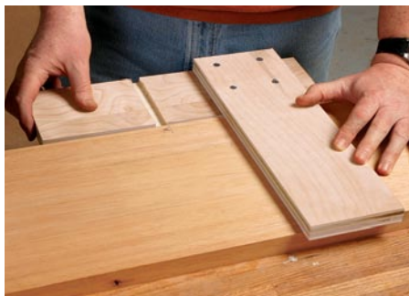
Right-angle jig ensures straight dados. Align the dado in the jig with the layout lines on the workpiece, then clamp the jig in place.
