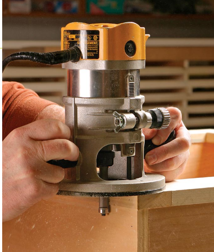
Trim face frames flush to case. The bearing on a flush-trimming bit is the same diameter as the cutter, allowing you to bring a frame flush to a carcass using a handheld router.
