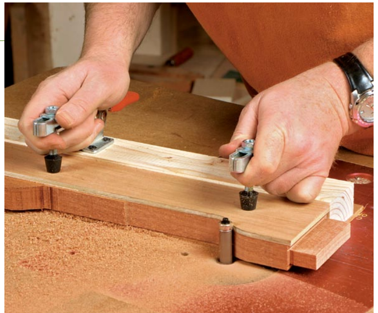
Create identical parts on the router table. Cut away most of the waste on the bandsaw first, then place the workpiece in a jig with the template on top (see drawing). The bearing will ride against the template, making an exact copy of the original. Cut with the grain, and reverse the workpiece in the jig (if possible) when the grain changes direction.
