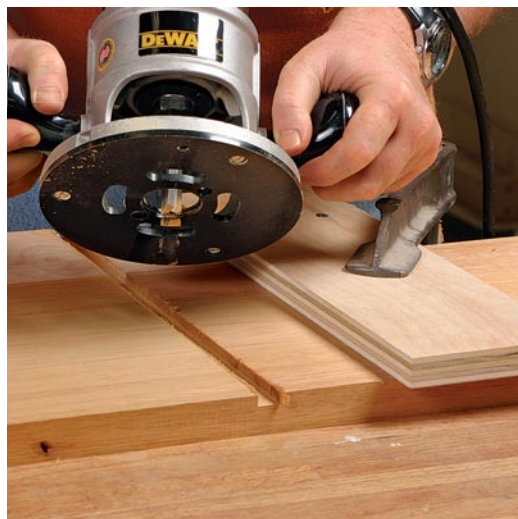
Work on this side of the fence. Then the bit's rotation will pull the router base against the jig's fence, ensuring an accurate cut.
