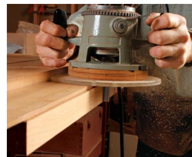
Router as jointer. With the help of a jig, you can clean up rough-sawn edges on large workpieces such as tabletops. Work from left to right.
