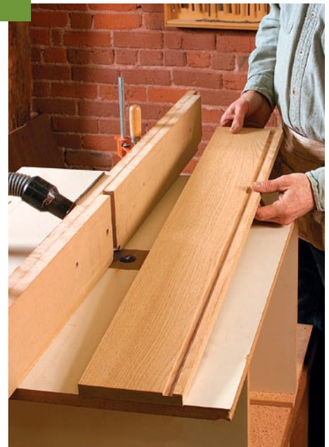
Grooves are best cut on the router table. For smooth cuts with little burning, take light passes, gradually raising the bit to full height.
