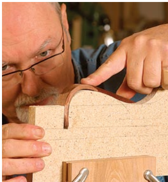
Check the first bend. Verify your accuracy by placing the first bend against the template.
