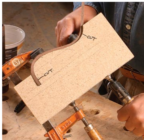
A setting jig. Often, the template for checking the curve also serves this role.
