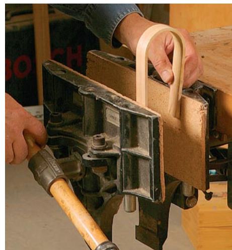
Held in a vise. You may be able to dry small parts by clamping them lightly in a bench vise.
