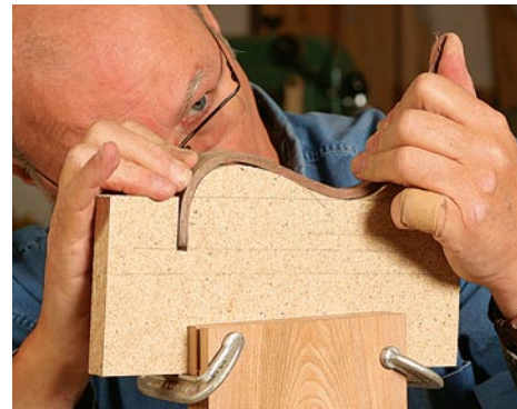
Right all around. Check the second bend against the template. By the way, this handle works on doors and drawers.
