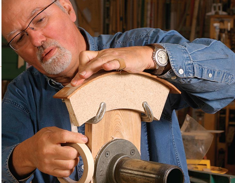
Clamp lightly. If the workpiece has not been bent sufficiently while being heated, firm clamping will not finish the job. A few clamps or even masking tape should be all you need.
