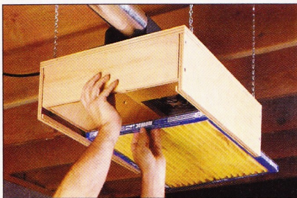
Grooves. The grooves allow you to easily slide the filter in and out, but they're positioned to provide an airtight seal.
