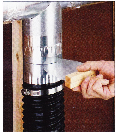
Sliding a shop-made blast gate in and out of a pipe turns the suction off (or on) at each tool.
