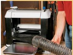
Helpful new features. The chute on the Delta (above) flips to allow the hose to connect to either side. The Craftsman 21759 (right) and DeWalt 735 blow their own chips into almost any container, without a dust collector attached.
