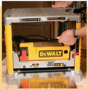
Managing snipe. When snipe is too extensive, it can't be corrected with sanding or scraping and must be cut off the end of the board. Some machines, like the DeWalt 734, have cutterhead locks built into the design. These locking devices reduce the amount of snipe.
