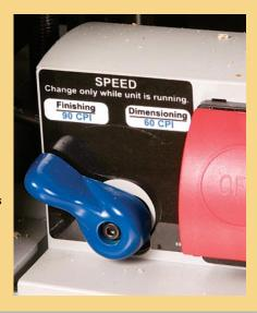
become on the surface of the board. Cuts per inch determines how close these cuts are.
