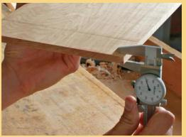
**Too much snipe?** If snipe is just a couple of thousandths of an inch deep, it can be worked out by sanding and scraping and is not a concern.
