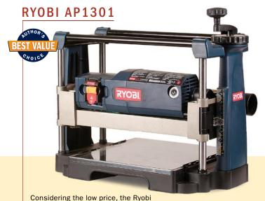
has an impressive amount of power. The lack of extension tables could lead to more snipe than the other machines, but I didn't find excessive snipe while planing an 8-in.-wide by 40-in.-long board. Add reasonably good dust collection (adjusts to blow chips out the back or hooks to a dust collector on the side) and the package becomes a great value for any shop.
