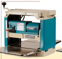
The Makita is a good performer with a lot of power. Blade changes are simple. Unlike the rest of the machines, one revolution of the crank handle does not move the cutterhead 1/16 in., making it awkward to intuitively change the depth of cut.
