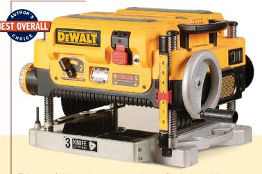
This powerful planer has a compact, low-profile design and leaves a great finish surface. It had no problem cutting 3/32 in. off an 8-in.-wide white-oak board. The side crank handle for height adjustment is awkward compared to the top-mounted models. There is good access to the knives for changing. Dust collection is quite good, but the hose attaches directly above the center of the outfeed table, which is slightly inconvenient if the hose isn't rigged out of the way.
