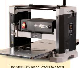
The Steel City planer offers two feed speeds, a three-knife cutterhead, good power, good dust collection, fast and easy knife changes, and moderate weight. All this adds up to a solid performer.
