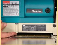
**How big a bite?** There are different ways to determine how much material will be removed. Delta's "Blade-Zero" device (left) pops up when the cutterhead is even with the top surface of the board; from there the depth of cut is set by turning the crank a measurable amount. On the Makita (center) a loose pin moves with the cutterhead against the top of the stock, giving a visual idea of how deep the cut will be. Other models have depth-of-cut indicators that give an exact measurement (right).
