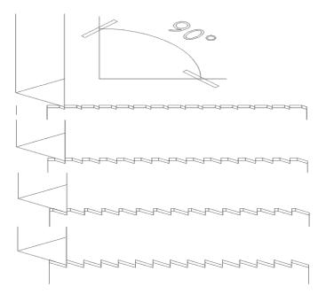
For shaping the teeth, I try slowly bring it to the next to the last diagram, leaving just a little bit of flat space on the top of the teeth. This helps me by serving as a guide to maintain the appropriate size of each tooth as I'm filing away. I stop there, and leave the remainder for the final sharpening.
