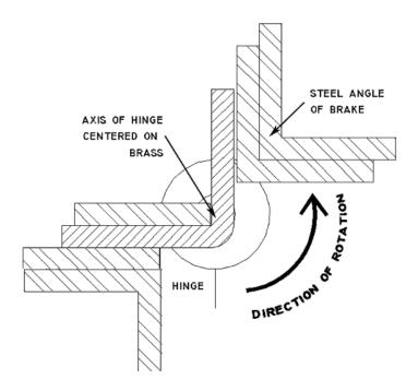
This configuration allows one to bend the brass easier, with more consistency, with less damage to the brass itself, and allow me to bend the brass a full 180 degrees, leaving only the thickness of the steel it is bent over. I can later use a hammer to close the brass completely over the saw blade. Many bending brakes cannot achieve this - getting you only about 120 degrees of bend, leaving too much hammer work, which means more potential for damaging the brass (at least for me).
