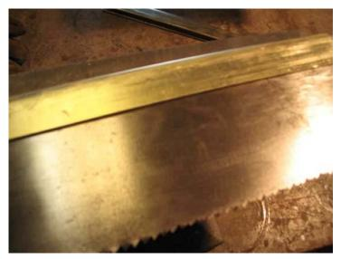
There it is - the back is installed. However - no matter how careful you are, there is bound to be some damage done by the hammer or bending or what not that you've done to it by this point:
