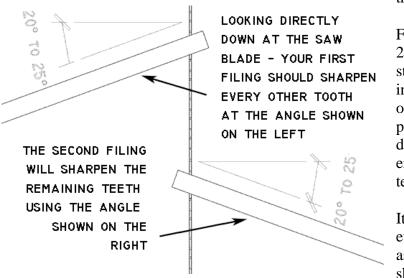
For backsaws. I use about a 20 to 25 degree angle. A steeper fleam angle results in a sharper saw, but also one that dulls quicker (on panel saws I use a 15 to 20 degree angle). You should end up with evenly shaped teeth, as below:
