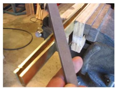
two thicknesses of brass, but thankfully it was only one that came out poorly enough to require it. On about half of the remaining, I used a disk sander to even up the edges:
