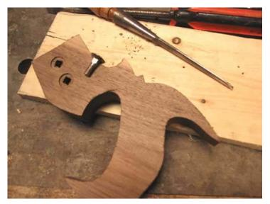
You must not skip this step. If you try to force them, the handle will crack - almost guaranteed. When the holes are all drilled, I test fit the handles:
