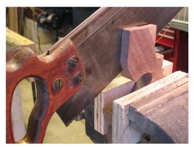
The photo to the left shows the depth of cut I made. You can use the intended blade as a guide, drawing its profile on the side of the handle blank at its desired location, and sawing to the depth it indicates.
