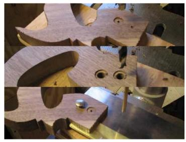
For the last hole I mounted the blade and got a standard high speed steel bit the width of the screw that I was using for the handle, then drilled the first hole through both the handle and the blade. Then, using a screw to make sure the blade didn't move and misalign the hole (see the bottom of the photo above) I drilled the final hole.
