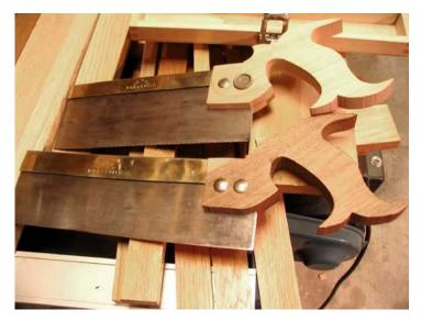
Don't over-tighten the screws yet - you need to be able to take the whole thing apart for the next step. You shouldn't tighten the screws fully until you are sure you will never have to take them apart again. This is a good time to make the final cut on the band saw - the portion just below the nuts. You can see the pencil line in the top saw where I was to make that cut.
