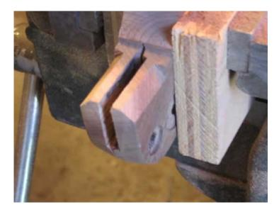
When finished shaping, I sand the handle starting with 80 or 100 grit sandpaper, finishing with 150 grit if I want to do any carving on the handles, or 220 grit if I don't. If I'm not going to do any carving on the handle, it's ready for the finish, which I'll cover in another segment.
