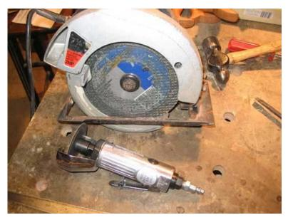
It's great for short cuts where the circular saw would be at a big disadvantage, though my air compressor can't keep up with it for longer cuts. In any case - if you use existing saw blades, they will probably need a bit of clean-up, and this would be the time to do the majority of that work as it is more difficult to do once you have the backs in place. I used a belt sander with 120
