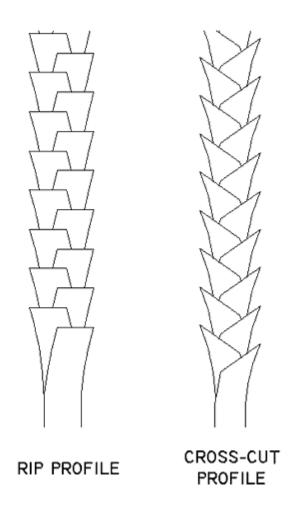
Dad always told me that you could slide a needle down the valley that forms between the teeth of a well-sharpened crosscut saw. I say this just to point out the slicing cut that it makes. Personally, I have used each for cutting dovetails - and I can't say I prefer either
