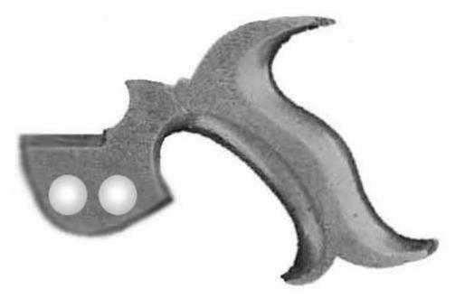
Also - the swoop of the handle at the bottom back can be "shortened" (for a lack of a better term) - this has the same basic effect. My best advice is to try it with a couple scraps first. Remember, a rough sawn blank like the one in the photo below should feel just a bit small and constricting in your hand. Rounding over the edges has the effect of making them feel a bit bigger, too.
