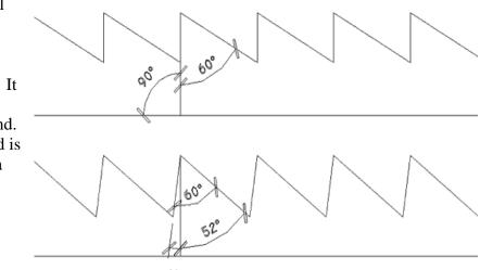
As shown in the above diagram, file the teeth at 90 degrees to the blade, using the same angle used in shaping the teeth above. Here's the real-world shot:
