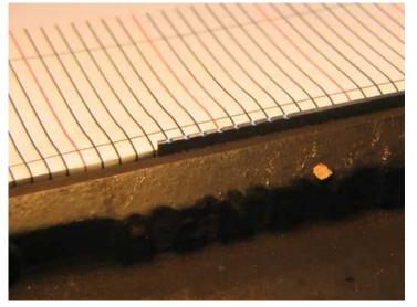
The photos I'm using are for a 9 PPI blade; so that you can see what I'm doing better than if I used the actual photos from the 15 PPI (or so) blades sharpened for these backsaws. The process is the same for either, however.
