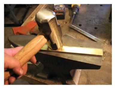
I had to be very careful that I brought the head of the hammer straight down on the brass, centering it right at the top of the back at the center of the radius of the curve, just like you see in the photo above. The mass of the large hammer made this easier, allowing me to lift it only about 4" or so above the brass, and bring it straight down. I worked the entire length of the back without the blade installed at about one inch increments, from front to back, flipping it
