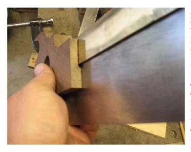
As I insert the blade into the handle, it begins to bind against the sides of the mortise, so I pull it out and pare more wood away until it slides in snugly. You can see in the mortise where the blade is binding on the wood, as it will be compressed slightly, and a bit darker. Be careful and don't force the blade into it's slot, as the way the grain of the wood works in this area it makes it easy to break off the corner, making the handle a complete waste. If I needed to make the
