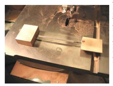
To initially shape the teeth, I work from one side only, and perpendicular to the blade. Trying to skip every other is difficult at best, and unnecessary at this point, as I'll finish sharpening them later by doing every other tooth. I'm not going to worry about the fleam angle (crosscut saws only) at this point, just getting the teeth properly shaped. Starting from flat, this will be the progression of the teeth as I file them (note - I'm showing a rip profile, but a crosscut would be similar):
