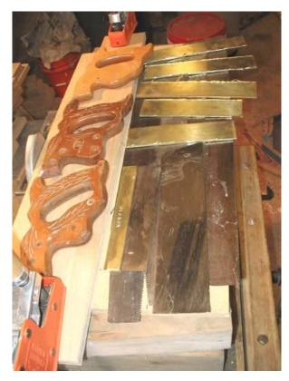
Now I have the steel and brass cut to rough size... It's time to get to it - and start making some saws! OK - not quite yet. There's one more step I must complete before I can actually start making saws. I need a way to make the initial bend of the back.
