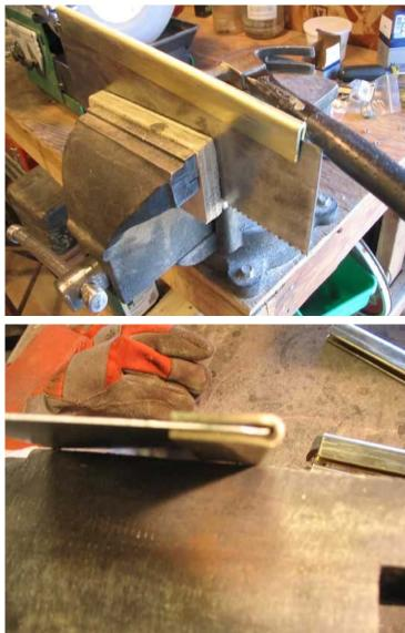
Notice the opening is straight for it's entire length... If you aren't careful, it's easy to introduce a bend into the brass that can be difficult at best to remove. It's best to try and minimize this by working slowly, keeping the bend as uniform as possible.
