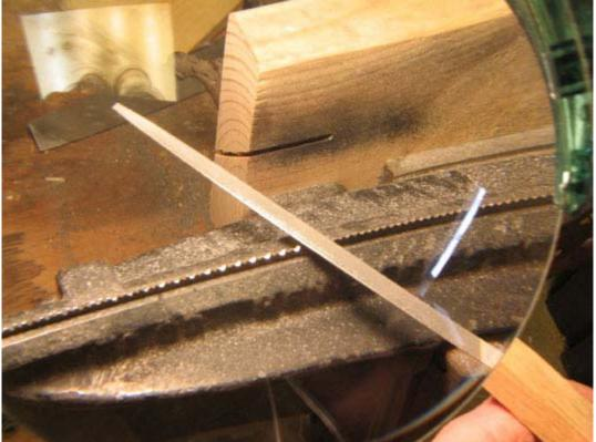
Because you are just introducing this angle to the filing, it may take an extra stroke to remove enough material to properly form the teeth. Just be careful, and watch that you don't remove too much that it makes it difficult to file the teeth from the other side. If you have to, just file a little, flip the saw file the other side, then repeat until you are finished. It's easier if you remove too little than if you remove too much.
