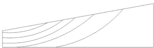
The blade, as shown in the diagram above, would be thickest at the right and the bottom, and vary in thickness between .010" and .015" or so. The tapering is done to help keep the saw from binding in its own cut. Many newer saws that you buy today will not have this feature.
