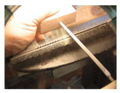
This last step usually only takes a light stroke or two of the file, just enough to remove the "flat" part left behind in the step above (see the "shaping" diagram). The flat will help you as a reference, filing the very last of it away should leave all of the points of the teeth in the same plane along the length of the saw, as seen in steps 4 and 5 of the diagram below - which goes through the entire shaping process:
