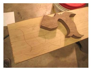
The grain of the wood in the handle needs to be oriented to there is a straight run of grain through the thinnest part of the handle, like you see in the photo above.
