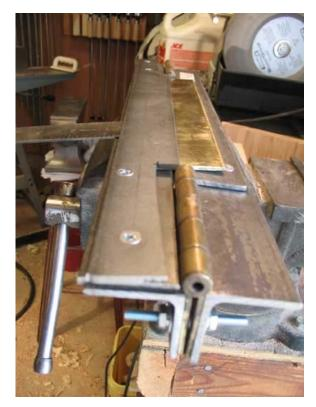
The entire affair is bolted together using #10 flat head machine screws, where the head of the bolt was made flush through using a countersinking bit. You'll notice the screws I used are much longer than necessary - that's because that's the size I
