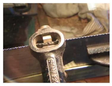
Using a saw set - notice the mark I've made on every other tooth with a marker:
