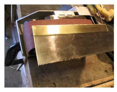
While you're sanding the back, the brass can get pretty hot - it's a good idea to keep a bucket of water handy to cool the blade off with, so it doesn't get too hot and begin to lose it's temper. Keep a towel or something handy to dry the blade off with when you're done, because you don't want the blade to start rusting again! For underneath the back, it's not as important to keep the steel from rusting a little bit. It might even be a good thing - a little bit of rust might help hold
