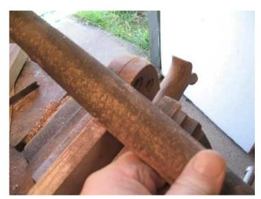
I also use a file to create a pair of reveals at the top of the handle where the back protrudes (photo on left)
