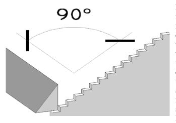
For rip-filed saws, you're nearly finished. All that's left is to run a file across every other tooth from one side, then flip the saw and run the file from the other direction on the remaining teeth. This is done so the filing is consistent from each direction, and any inconsistencies that are created by your technique are repeated in an opposite and equal manner. The angle should be the same one chosen previously (the lower is the less aggressive pitch):
