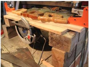
The saw's base is simply screwed to a piece of particle board. A piece of plywood screwed to the "table" serves as a fence, and I just clamp the whole affair to my bench, as you can see. If you do this, you'll probably need to wear a pair of gloves while cutting the steel, both because of the sharp edges and possibly because of the heat (bigger issue when cutting the brass than the steel). Keep an open pail of water handy to dunk the steel into to keep it from getting too hot. Make sure
