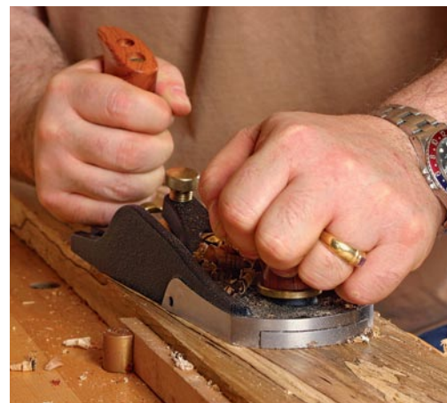
Low angles for smoothing spalted wood. Spalted wood is very soft, so you need a low-angle blade to slice through it with minimal compression.
