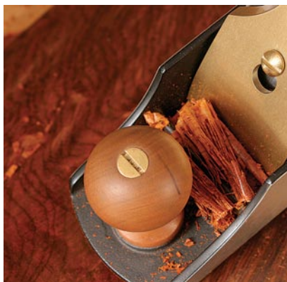
High blade angles. Woods such as tiger maple cut best at about 55° (top), while cocobolo (above) should be worked with the blade cutting at 60° to 65°.
