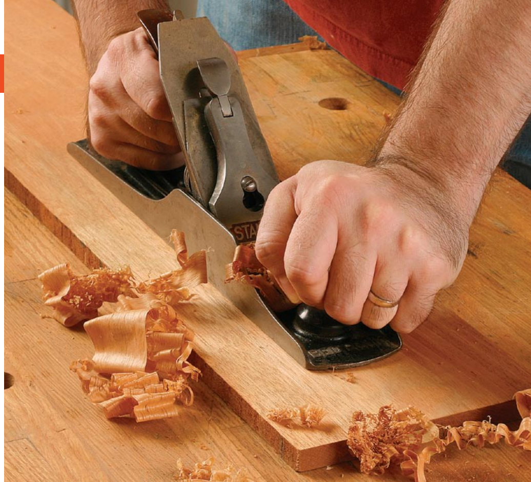
A different angle for different species. Easily worked boards of low-density hardwoods such as this piece of mahogany work best with the blade at a medium angle of around 45°.
